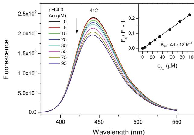
**Fig. 5** Fluorescence spectra of norfloxacin (10 μM) at pH 4.0 titrated with HAuCl<sub>4</sub>. The arrow represents increasing Au concentrations. Inset: Stern-Volmer plot for the fluorescence at 442 nm, and linear fit with the Stern-Volmer constant  $K_{SV} = 2.4 \times 10^3 \text{ M}^{-1}$  (Eq. 3)
