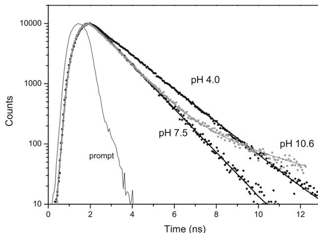
**Fig. 8** Intensity decays of norfloxacin at pH 7.5, 4.0, and 10.6 (TCSPC data). Excitation at 330 nm. Emission at 407 nm (pH 7.5 and 10.6), and 440 nm (pH 4.0)
