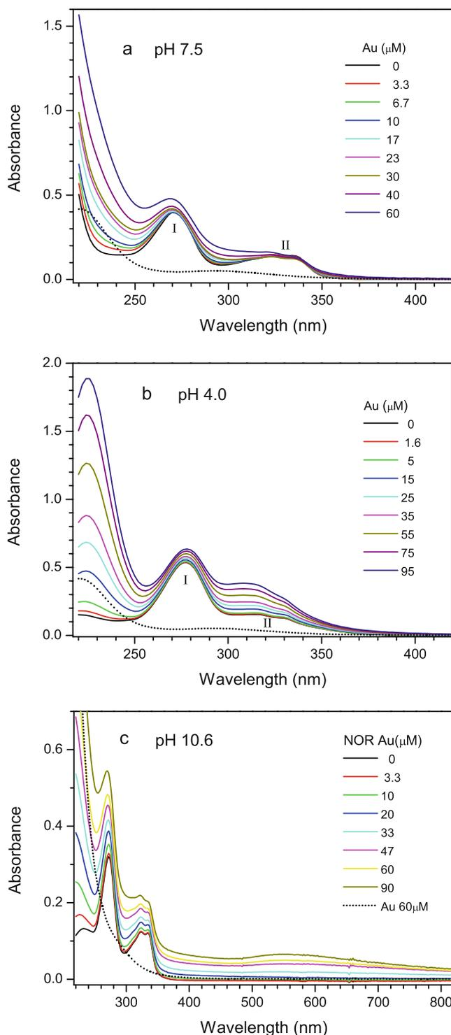
**Fig. 3** UV-visible absorption spectra of norfloxacin (10  $\mu\text{M}$ ) titrated with  $\text{HAuCl}_4$  at (a) pH 7.5, (b) pH 4.0 and (c) pH 10.6. The spectrum of  $\text{HAuCl}_4$  appears in the three figures as dotted lines (20  $\mu\text{M}$  in a and b; 60  $\mu\text{M}$  in c)
