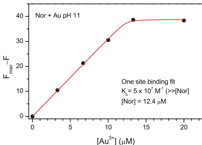
**Fig. 7** Fluorescence change of NF at 420 nm, pH 10.6, upon  $\text{HAuCl}_4$  titration. The line represents the one-site binding least squares fit using Eq. (2) with  $K_b = 5 \times 10^7 \text{ M}^{-1}$  ( $\gg [\text{Nor}]$ ) and  $[\text{Nor}] = 12.4 \mu\text{M}$
