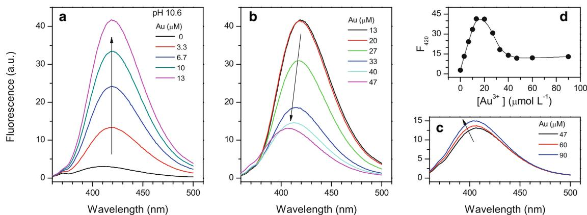
**Fig. 6** Fluorescence spectra of NF at pH 10.6 and different  $\text{HAuCl}_4$  concentrations: **a** from 0 to 13  $\mu\text{M}$ ; **b** from 13 to 47  $\mu\text{M}$ ; **c** from 47 to 90  $\mu\text{M}$ . The arrows indicate increasing  $\text{Au}^{3+}$  concentrations. **d** is a plot of the fluorescence intensity at 420 nm versus  $\text{Au}^{3+}$  concentration
