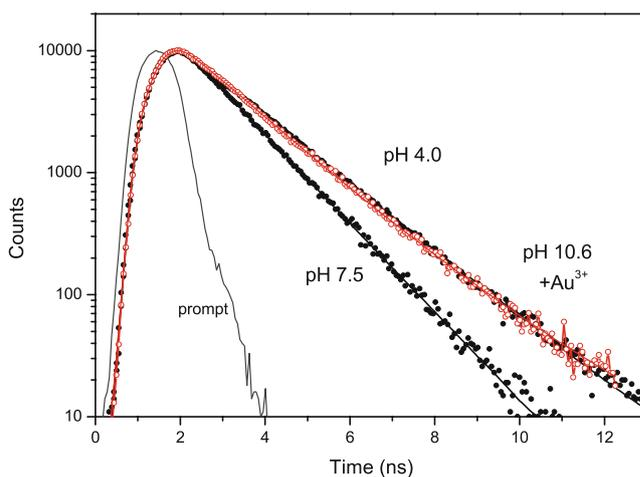
**Fig. 9** Decay of  $Au^{3+}$ -norfloxacin fluorescence at pH 10.6 (empty dots connected by straight line) compared with the decays of pure NF at pH 7.5, 4.0.  $[Au^{3+}]:[NF]=1.3$ . Excitation at 330 nm; emission at 420 nm (pH 10.6), 407 nm (pH 7.5), and 440 nm (pH 4.0)
