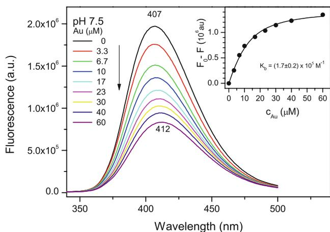
**Fig. 4** Fluorescence spectra of norfloxacin (10 μM) at pH 7.5 titrated with HAuCl<sub>4</sub>. The arrow represents increasing Au concentrations. Inset: fluorescence changes at 407 nm as a function of Au concentration, and the one site binding (Eq. 2) least squares fit with  $K_b = 1.7 (\pm 0.2) \times 10^5 \text{ M}^{-1}$
